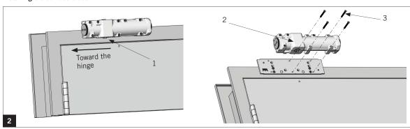
NOTE: Orient pinion (1) closest to hinge.
