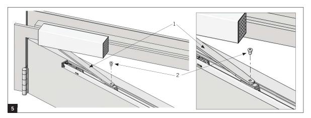
**5.1** Align the arm (1) with the hold open slide shoe in the track channel.
